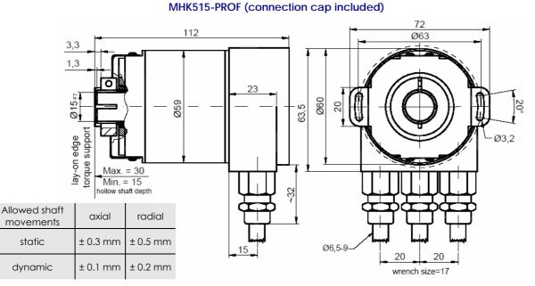
Shaft diameter can be reduced at 12mm, 10mm or 8mm by reduction ring (by inserting them into the hollow shaft)
